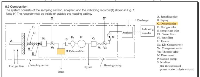
Note (5) The converter is installed at Ka or Kb. Ka may be outside the casing
